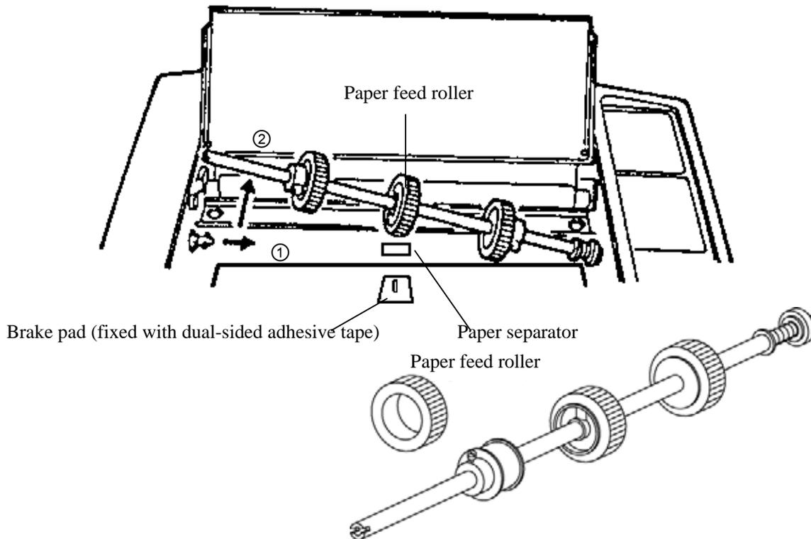
Grasp the paper separator (with plastic part) at both ends and pull it out. To install, reverse the procedure.
